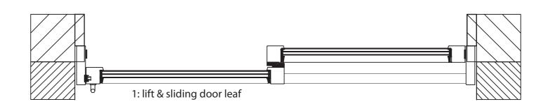
Standard: opening inwards - 1: lift & sliding door leaf runs inside Our systems with flat threshold are wheelchair accessible.
